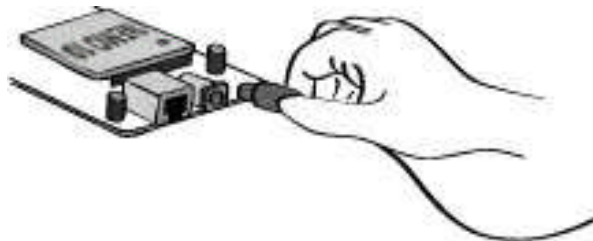
Figure 2-5 Connecting the power to the test bed
